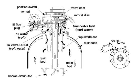
To begin a regeneration, the electronic timer energizes the circuit to the valve motor. The valve motor rotates the rotor and disc and the valve cam until the position switch lever drops, to open the motor circuit and position the valve in FILL. As the rotor and disc rotates, the port opens for SOFT water fill through the venturi. Fill flow continues to the brine valve, and into the salt storage tank. Soft water is still available to the house lines.
